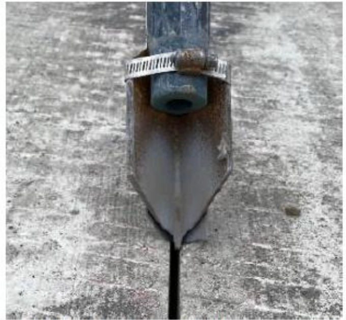
Figure 1 Media Blast Alignment Fixture
