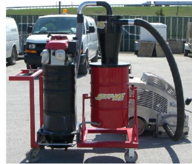
Figure 4 Photo of Early Entry Saw Vacuum Pickup Equipment
