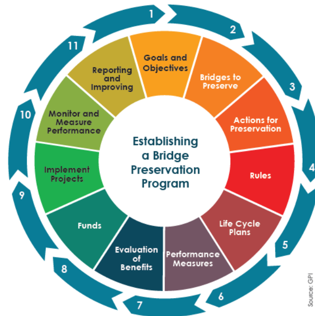
Figure 15. Steps for establishing a bridge preservation program.
