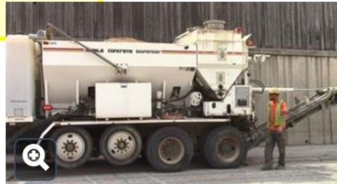
Volumetric proportioning of 3U18 with mobile mixer
