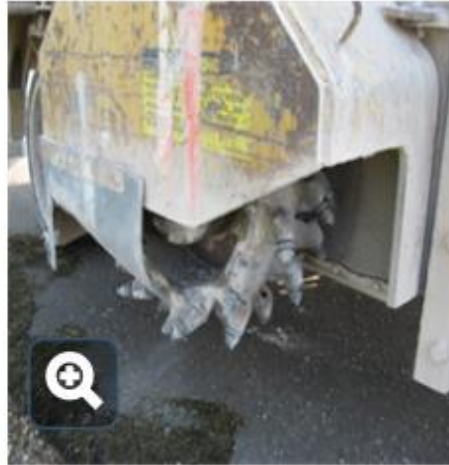
Carbide-tipped Cold Milling Head
