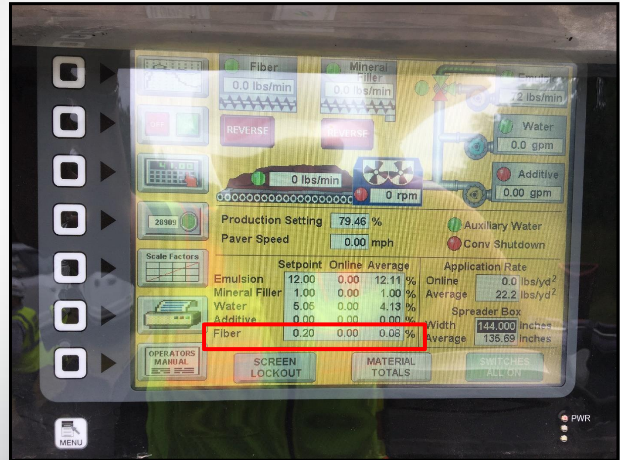
Fiber Dispenser with integrated rate indicator
